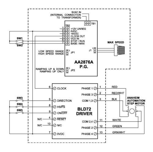
Power Requirements: 105 - 125VAC, 50 - 60Hz Logic "1" (open) - Motor current on Motor On/Off: (Terminal 9) Logic "0" - Motor Current Off TTL-CMOS Compatible Control Inputs: (Terminals 5, Logic "1" = OPEN 6, 8, 9) 3.5 to 5.0 V Logic "0" = 0 to 0.8 V Logic "1" (open) - Clockwise Direction Control: (Terminal 5) Logic "0" - Counterclockwise **Operating Temperature:** 0° to 60° C
